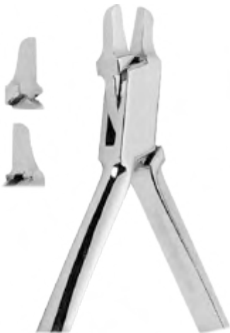
4425 Tweed (Angle) arch bending pliers - short - Pliers with beaks (10 mm.) designed for convenient handling of square or rectangular wires the blades are parallel at 0,5 mm. (.020") pliers' opening.
